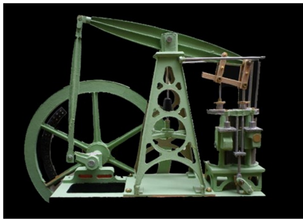
This is a model of the beam engine made by Eric Shaw and on display at our museum.
